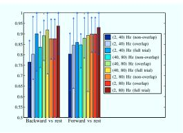
Figure 4. **Classification accuracy:** The figure shows the average test accuracy and test accuracy range across blocks for both binary classifiers (forward vs rest and backward vs rest) and three frequency ranges (2-40, 40-80 and 2-80 Hz).
