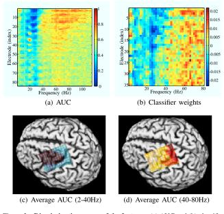
Figure 3. **Discriminative power of the features**: (a) AUC and (b) classifier weights per electrode and frequency bin, (c) average AUC per electrode for low-frequency band and (d) average AUC per electrode for high frequency band for moving backward vs resting. A similar figure was obtained when comparing move forward vs rest and it is omitted. Refer to Fig. 2 for the subject's brain with an overlay x-ray of the electrode grid.
